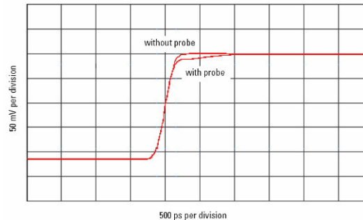
TDT measurement at receiver with and without probe load for 250 ps rise time
